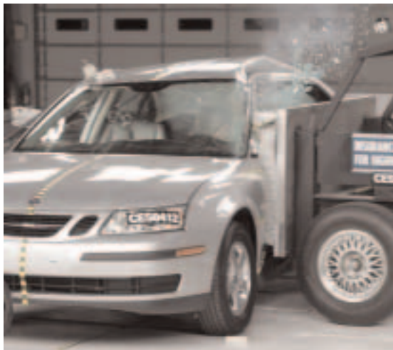
The test represents what happens when a passenger vehicle is struck in the side by a pickup truck or SUV.
