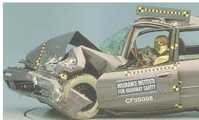
1995 MITSUBISHI GALANT Poor performance: major intrusion into the occupant compartment
