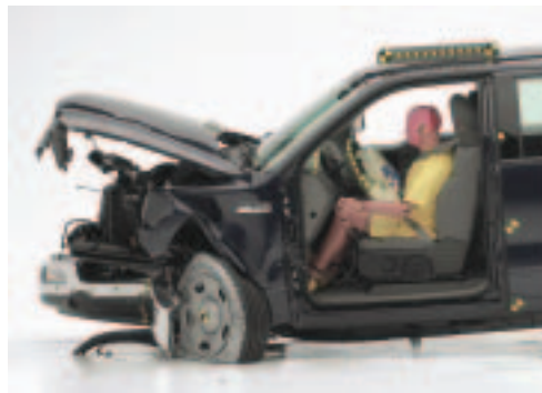
2004 FORD F-150 Good structural performance: Occupant compartment remained intact
