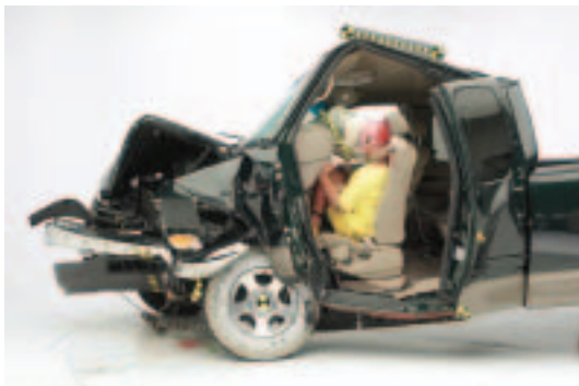
2001 FORD F-150 Poor structural performance: Massive collapse of the occupant compartment
