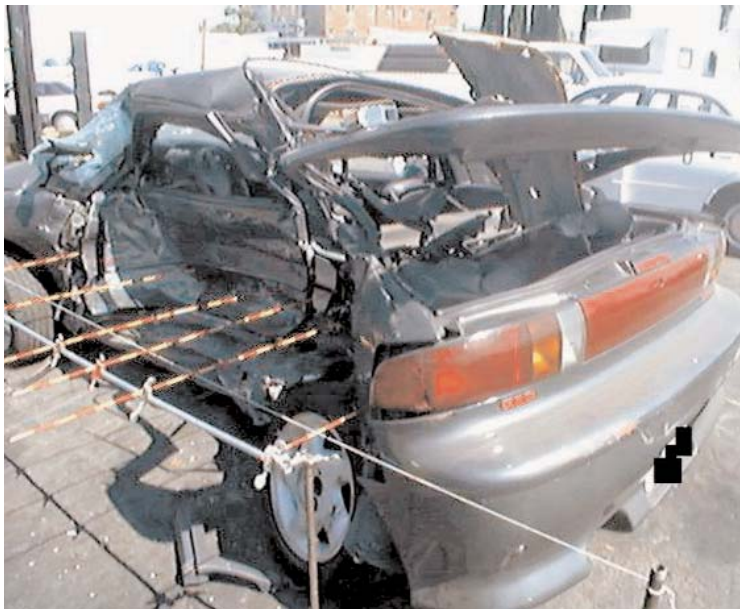
Head injuries are a leading cause of occupant deaths in side impacts. For example, the 23-year-old driver of this car died when his head was struck by the intruding front end of a pickup truck. See Attachment 3 for more examples.
