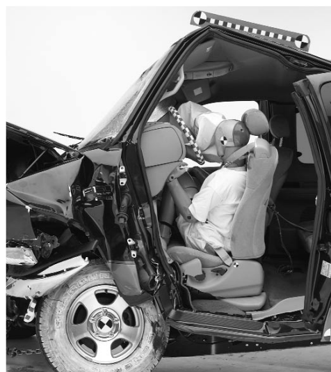
FORD F-150: The driver seat pitched forward while the instrument panel and steering column moved back. This severely compromised the driver space.
