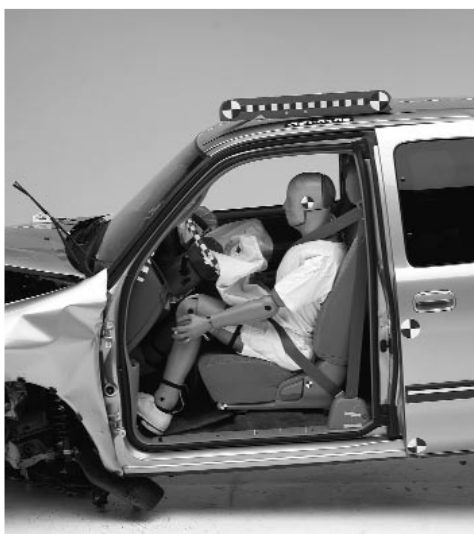
TOYOTA TUNDRA: The space around the driver dummy was maintained well during the frontal offset crash test at 40 mph.
