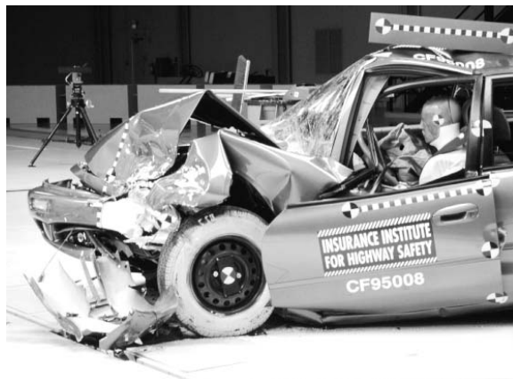
1995 Mitsubishi Galant rated poor for structural integrity. Survival space wasn't maintained well in 40 mph offset test.
