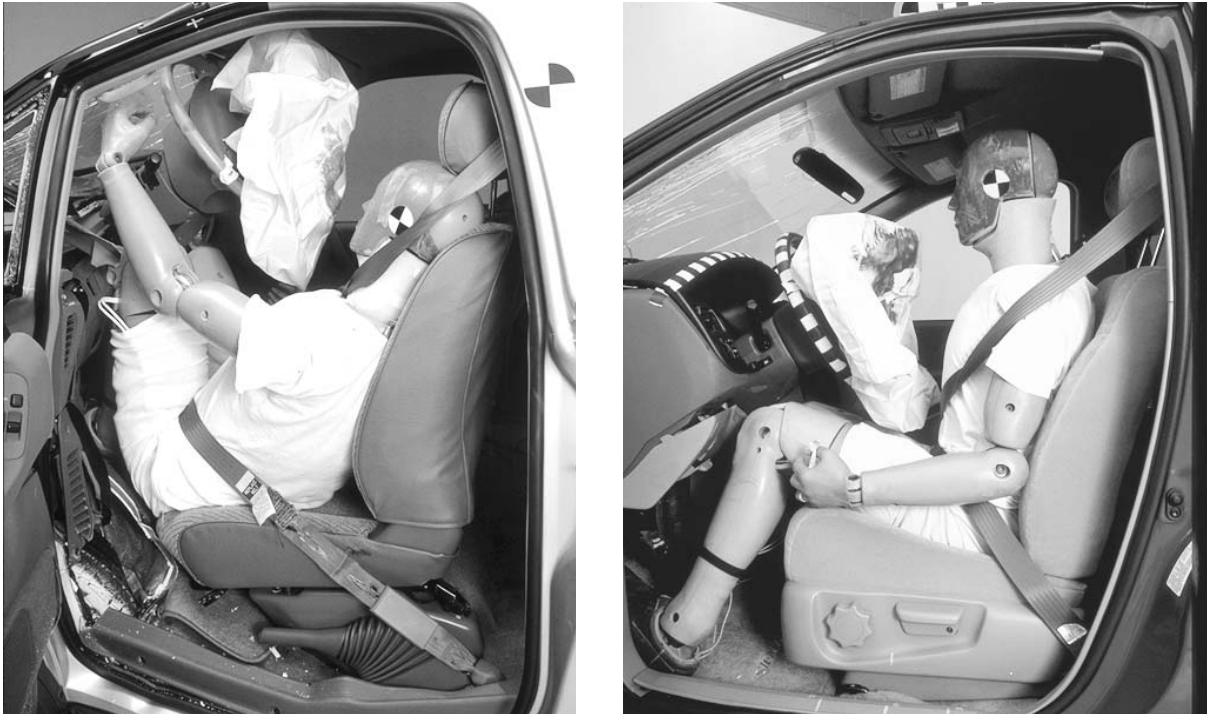
1996 Toyota Previa (left) and 1998 Toyota Sienna (right) after 40 mph frontal offset crash tests
