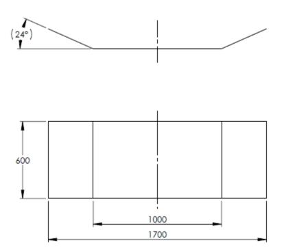
Figure 5. Bumper Cladding
