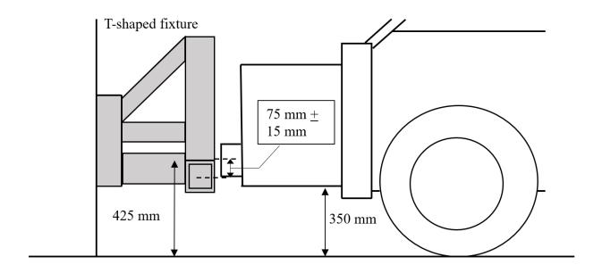
Figure 1B. Lateral barrier alignment
