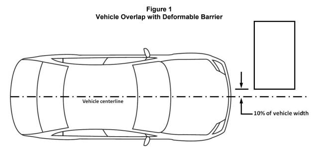
The vehicle is accelerated by the propulsion system at an average of 0.3 g until it reaches the test speed and then is released from the propulsion system 25 cm before the barrier. The onboard braking system, which applies the vehicle's service brakes on all four wheels, is activated 1.0 second after the vehicle is released from the propulsion system.
