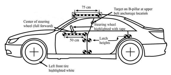
The head restraints are removed from the front seats, and the front right passenger frontal and side curtain airbags are deactivated (if necessary) to prevent these components from obstructing camera views. The airbags are deactivated by inserting an appropriately sized resistor in place of the connection to each airbag.
