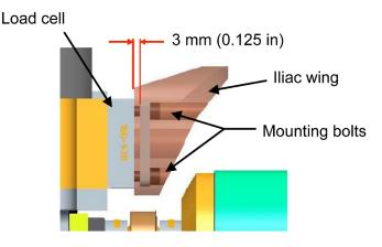
Figure 2 Superior-Inferior View of Iliac Load Cell and Iliac Wing (Top Photo) and Lateral-Medial View of Load Cell (Bottom Photo)
