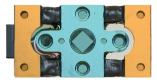
Note the normal gap between the iliac wing and center of the load cell. Tightening of the attachment bolts causes the ends of the load cell (orange highlight) to creep into the wing. Over time, there is sufficient creep (about 2 mm) for the wing to load the center of the load cell (blue highlight). This allows an externally applied force to bypass the correct load path.
