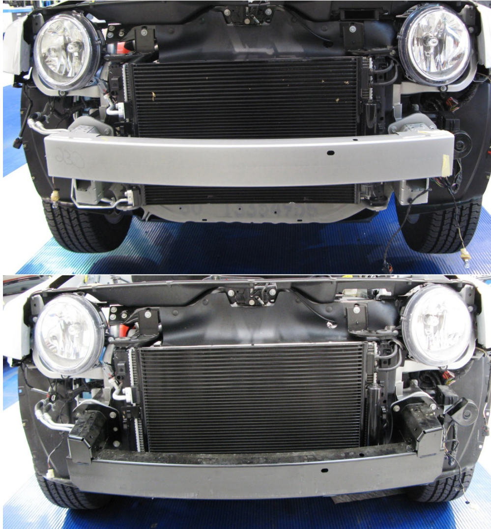
Figure 7 Jeep Patriot Front Bumper Modification – Original Equipment (top), Modified (bottom)
