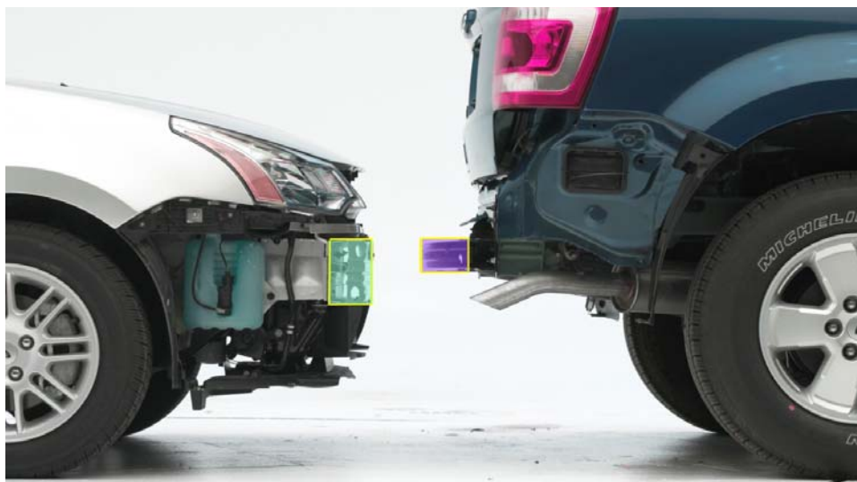
Figure 4 Modified SUV Bumper Location – Focus Front (left), Escape Rear (right)
