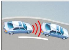
forward collision warning and auto braking
