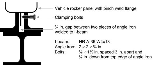
Figure 2 Rocker Panel Support System Attached to Vehicle Outboard (top) and Inboard (bottom)
