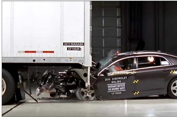
56 km/h, 50 percent overlap tests with 2007 Vanguard trailer (left) and 2011 Wabash trailer (right)
