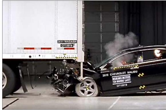
56 km/h, full-width tests with 2007 Hyundai trailer (left) and 2011 Wabash trailer (right)
