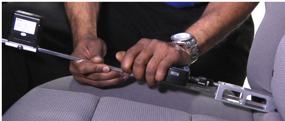
Figure 4. Measuring lower anchor attachment force.
