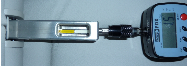
Figure 5. Force tool slider fully engaged on anchor.
