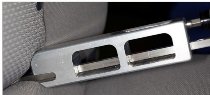
Figure 2. Initial position of force tool slider, with seat cushion just touching top and bottom of front surface of force tool slider.
