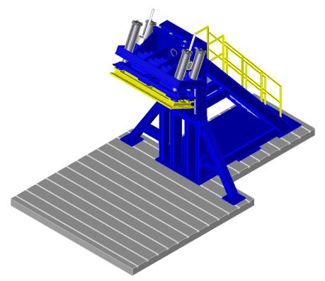
Figure 3 MGA Roof Crush Test System
