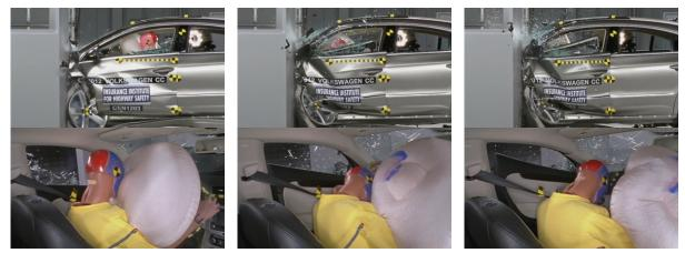
During the crash, the dummy's head barely contacted the frontal airbag before sliding off the left side. There were no other countermeasures to prevent head contact with hard structures forward of the airbag.
