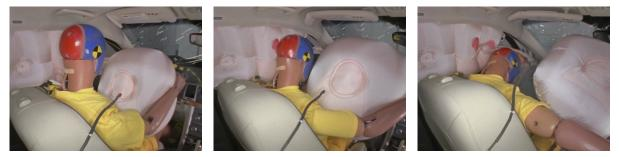
During the crash, the dummy's head missed the frontal airbag entirely, and there were no other countermeasures to prevent head contact with hard structures forward of the airbag.
