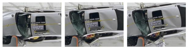
The outboard motion of the dummy, with respect to the vehicle interior, combined with the absence of a side head protection airbag allowed the most of the dummy's head to move outside of the precrash window plane.
