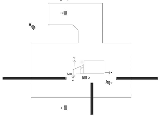
Figure 5B Onboard High-Speed IDT Camera Positions
