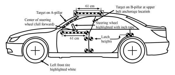
steering wheel center in the longitudinal direction. To determine vehicle alignment with the barrier at impact, inch tape is placed at 24 and 26 percent of vehicle width. The steering wheel and the leading edge of the dash are highlighted with inch tape, and the left front tire is highlighted with white paint.
