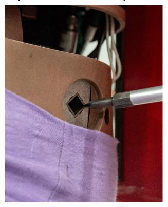
Figure 5b CMM point 2: Rear base of neck along dummy centerline
