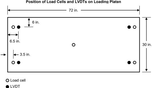
Figure 4 Position of Load Cells and LVDTs on Loading Platen
