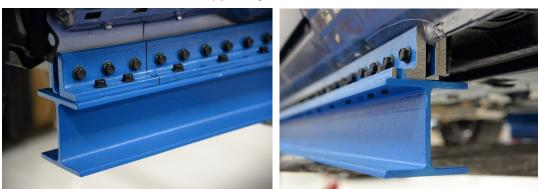
Figure 1 Rocker Panel Support System - Attached to Vehicle
