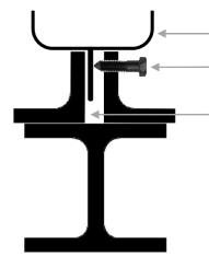
Vehicle rocker panel with pinch weld flange
