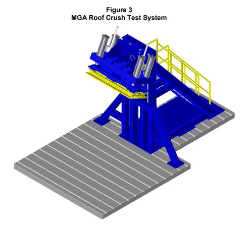
Two HR A-36 W10x88 I-beams are mounted on the bed plate perpendicular to the longitudinal axis of the platen. The vehicle, with attached rocker panel support system, is placed on these beams. The vehicle is adjusted so that:
