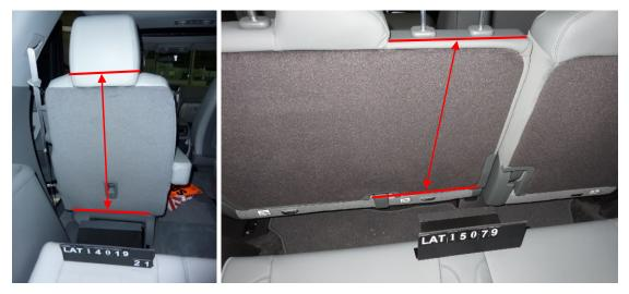
Figure 10. Seatback length, measured on rear of seatback between top- and bottom-most points of seatback.
