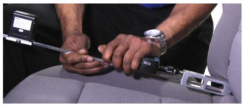
Figure 6. Measuring lower anchor attachment force.
