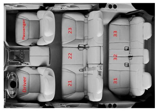
Figure 1. Designation of vehicle seat positions.
