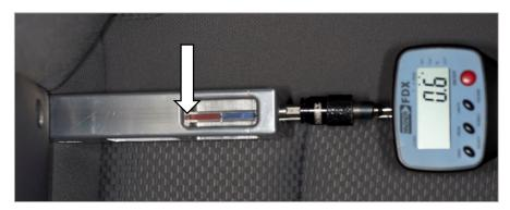
Figure 5. Depth within bight is estimated from color visible at front edge of viewing window, which is red (2 to 4 cm) in this example.
