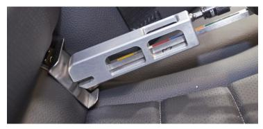
Figure 4. Initial position of force tool slider, with the tunnel adaptor just touching top and bottom of front surface of force tool slider.
