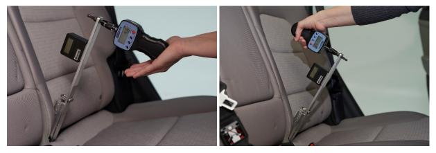
Figure 9. Measuring lower anchor clearance angle in push (left) and pull (right) mode.
