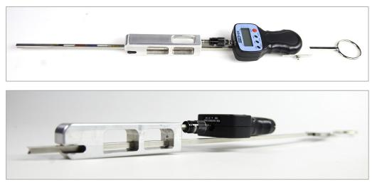
Figure 2. Attachment force tool used to measure depth of lower anchor within seat bight and anchor attachment force.
