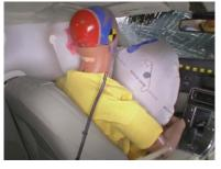
The dummy's head contacted the frontal airbag but slid left into a gap providing no support for the head. This gap mainly was due to the narrow, asymmetric frontal airbag. There were no other countermeasures to prevent head contact with hard structures forward of the airbag.
