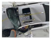
The outboard motion of the dummy, with respect to the vehicle interior, combined with the absence of a side head protection airbag allowed the most of the dummy's head to move outside of the precrash window plane.
