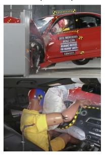
The airbag provided significant support to the head early in the crash, but the dummy continued to move laterally outside of the original extended perimeter of the airbag, and there was little airbag volume between the dummy's head and interior structures. The dummy contacted the roof rail during rebound. There were no other countermeasures to prevent head contact with hard structures forward of the airbag.
