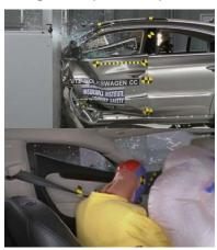
The dummy's head barely contacted the frontal airbag before sliding off the left side and undergoing additional forward excursion. There were no other countermeasures to prevent head contact with hard structures forward of the airbag.
