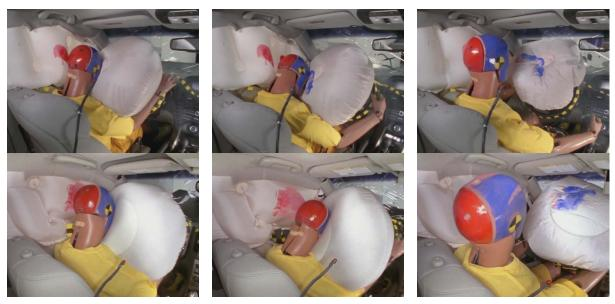
The dummy's movement in these tests was well controlled. The dummy's head loaded the frontal airbag and stayed in contact with the airbag within its original extended perimeter until the dummy rebounded in the rearward direction.
