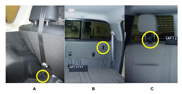
Figure 11 Potentially confusing hardware includes cargo tie-down points (A), seatback latches (B) and tether routers (C).
