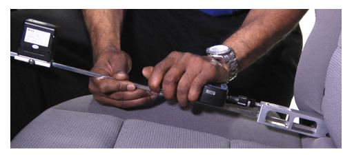
Figure 6. Measuring lower anchor attachment force.
