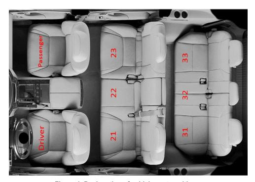
Figure 1. Designation of vehicle seat positions.
