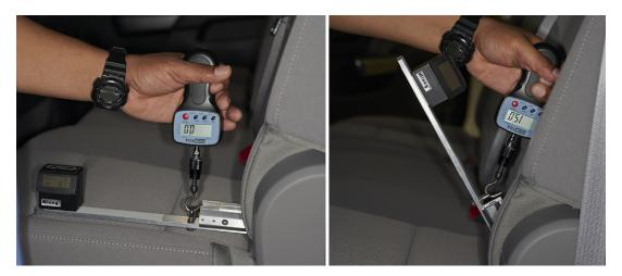
Figure 9. Measuring lower anchor clearance angle.
