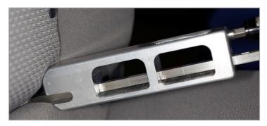
Figure 3. Initial position of force tool slider, with seat cushion just touching top and bottom of front surface of force tool slider.
