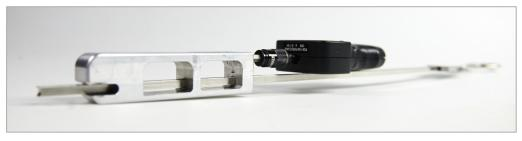
Figure 2. Attachment force tool used to measure depth of lower anchor within seat bight and anchor attachment force.
