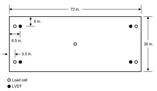
Figure 5 Position of Load Cells and LVDTs on Loading Platen
