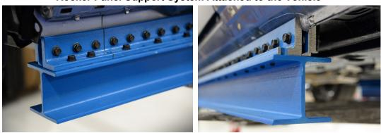
Figure 1 Rocker Panel Support System Attached to the Vehicle
