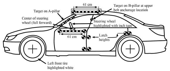
steering wheel center in the longitudinal direction. To determined vehicle alignment with the barrier at impact, inch tape is placed at 24 and 26 percent of vehicle width. The steering wheel and the leading edge of the dash are highlighted with inch tape, and the left front tire is highlighted with white paint.
