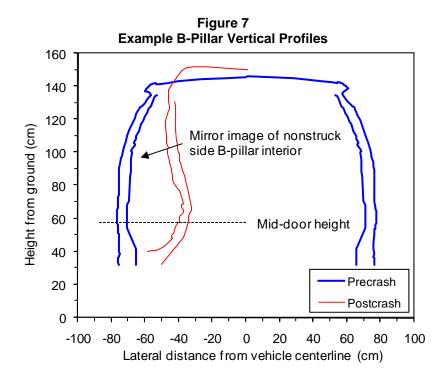
**Coordinate system definition** – A right-handed, three-axis orthogonal coordinate system is used for these measures: longitudinal (front to rear is positive), lateral (left to right is positive), and vertical (bottom to top is positive).
