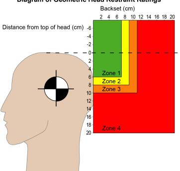
Figure 1 Diagram of Geometric Head Restraint Ratings
