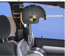
Figure 8 Measuring Backset for BioRID Set-up
