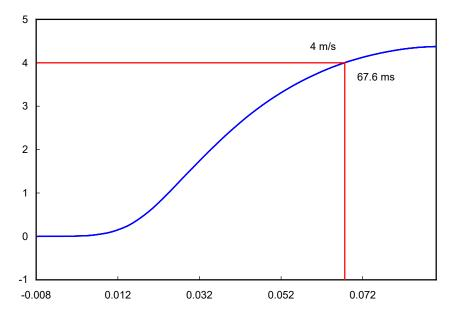
Step 7. Subtract the time recorded in step 6 from 70 ms. Add the difference to the time indexed head contact time from step 3. The resulting value will be the official head contact time (HCT) used for evaluation.
