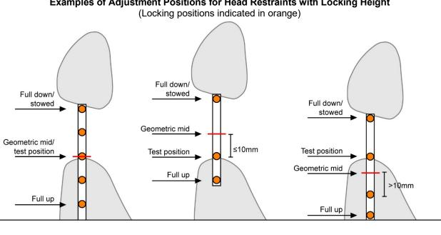
Figure 7 Examples of Adjustment Positions for Head Restraints with Locking Height
