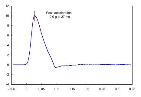
Step 4. Filter sled acceleration data to CFC 180. Integrate from the last time the acceleration passes through zero at the beginning of the trace until the first time the acceleration passes through zero at the end of the trace.
