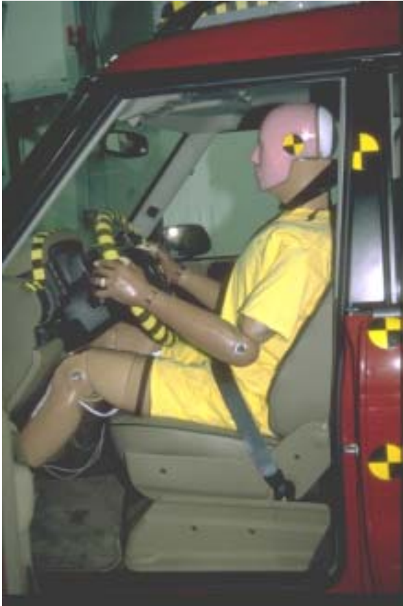
Figure A1 50th Percentile Hybrid III Male ATD Positioned in 1999 Land Rover Discovery Series II Prior to IIHS Frontal Offset Crash Test; Seat Positioned According to FMVSS 208 Specifications
