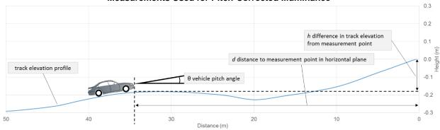
Figure 1 Measurements Used for Pitch-Corrected Illuminance
