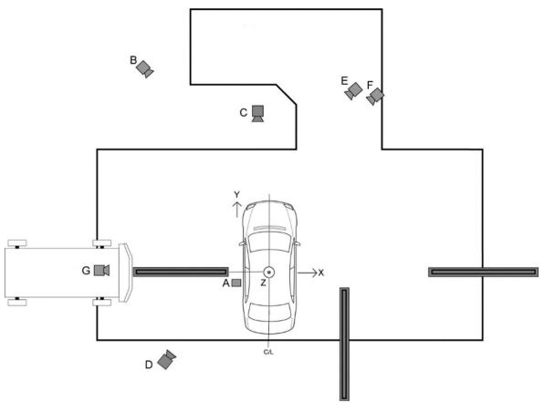
Figure 6B Onboard High-Speed IDT Camera Positions
