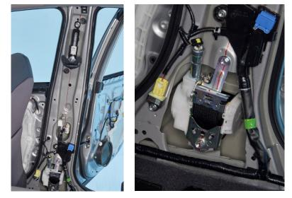
Figure 8 Example of Interior B-Pillar and Crash Tensioner Profile Measure — Precrash
