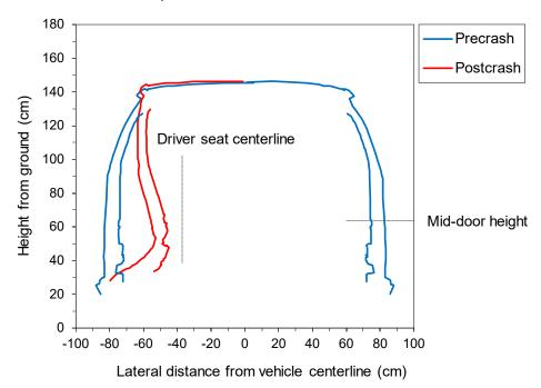
Figure 7 Example B-Pillar Vertical Profiles
