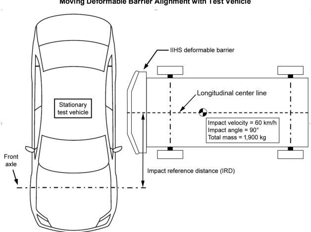
Figure 1 Moving Deformable Barrier Alignment with Test Vehicle
