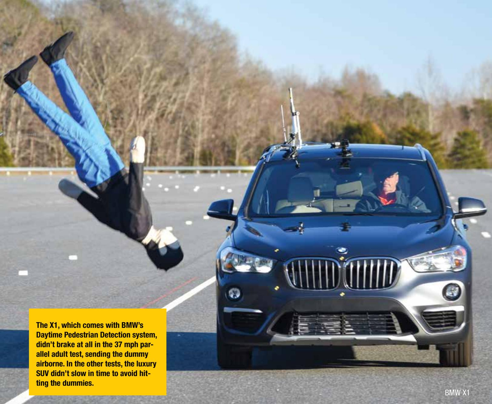
**The X1, which comes with BMW's Daytime Pedestrian Detection system, didn't brake at all in the 37 mph parallel adult test, sending the dummy airborne. In the other tests, the luxury SUV didn't slow in time to avoid hitting the dummies.**
