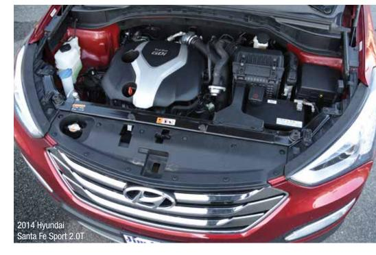
Hyundai and Kia vehicles with a 2.0-liter turbocharged engine have the highest frequency of noncrash fire claims, followed by 2.4-liter engine models. NHTSA is investigating both of these Theta II engines.
