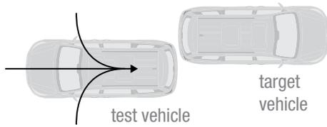
This scenario simulates backing out of a parking space toward a stationary vehicle. Test runs include reversing straight back and from the left and right toward the target. If autobrake fails to prevent a collision, the test vehicle will strike the corresponding portion of the target vehicle bumper with an overlap of 16 inches.
