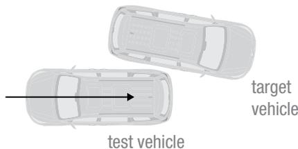
This scenario simulates backing toward the side of an adjacent stationary vehicle. The test involves reversing straight back toward the target vehicle parked at a 10-degree angle to the test vehicle.
