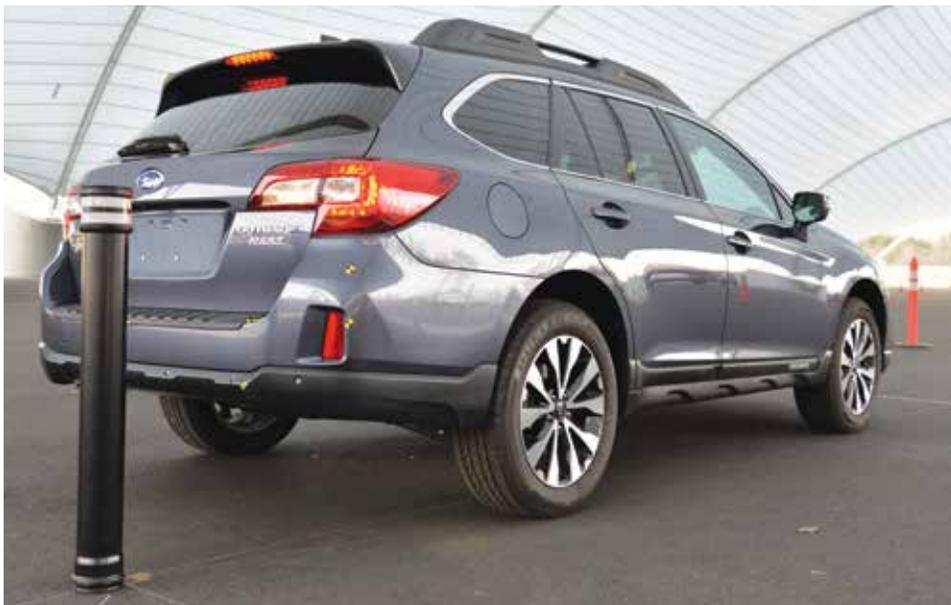
Left: One of the tests in the Institute's new rear crash prevention assessment evaluates a rear autobrake system's ability to stop a reversing car from striking a pole — a common mishap that can lead to pricey damage to bumpers, fenders, lift gates and lights.
