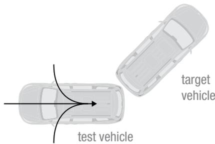
This scenario involves reversing out of a parking space toward a stationary vehicle. Test runs include reversing straight back and from the left and right toward the target. If autobrake fails to intervene, the corner of the test vehicle's bumper will strike the center of the target vehicle bumper.
