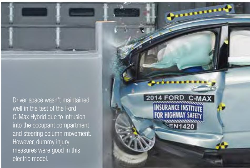
Driver space wasn't maintained well in the test of the Ford C-Max Hybrid due to intrusion into the occupant compartment and steering column movement. However, dummy injury measures were good in this electric model.
