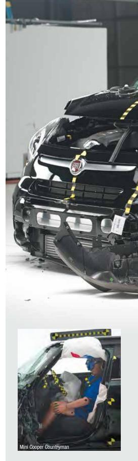
The Mini Cooper Countryman's safety cage held up well, and the safety belts and airbags worked as they should to control the test dummv's movement.
