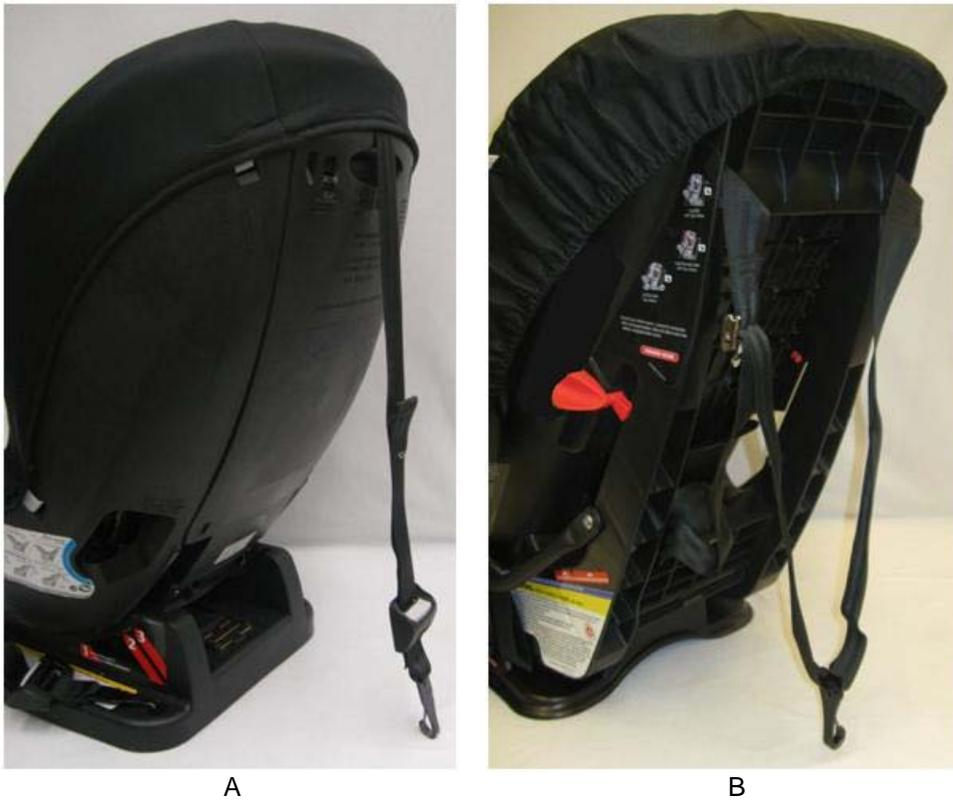
**Figure 4** Evenflo Triumph child restraint with a single-strap tether (A) and Britax Marathon 70 child restraint with a v-shaped tether (B)
