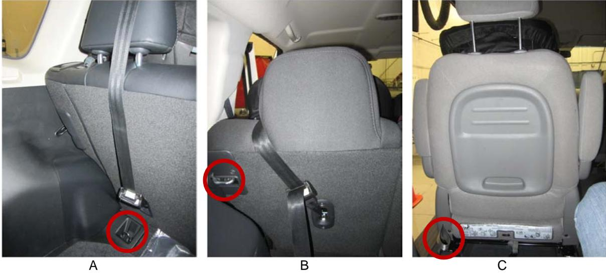
**Figure 3** Potentially confusing hardware includes cargo tie-down points (A and B) and webbing loops (C).
