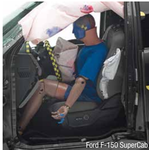
There was extensive occupant compartment intrusion in the Ram 1500 (left), resulting in a poor rating for structure. In contrast, survival space was well-maintained in the Ford F-150 (right).
