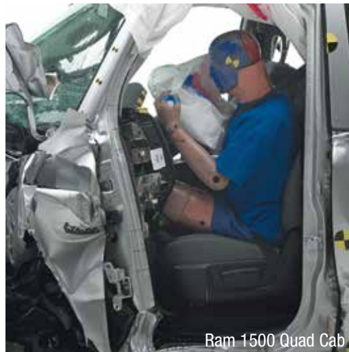
There was extensive occupant compartment intrusion in the Ram 1500 (left), resulting in a poor rating for structure. In contrast, survival space was well-maintained in the Ford F-150 (right).
