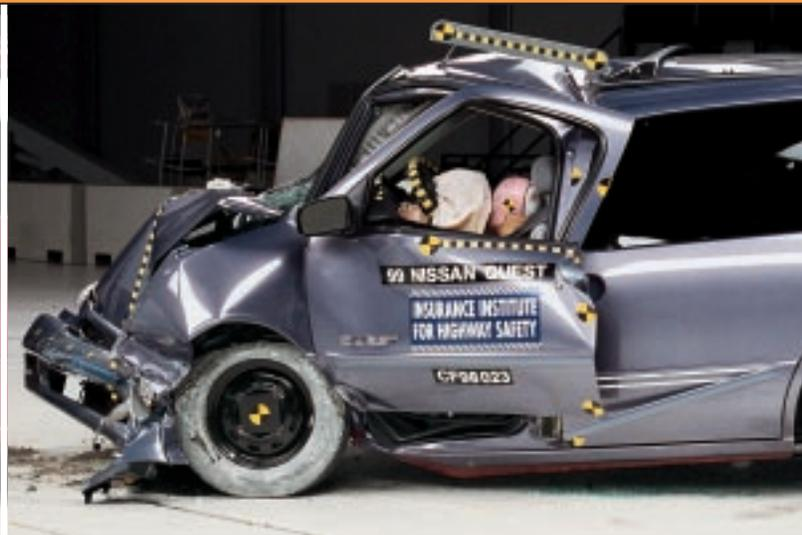
**Complementary tests:** The Institute's crashworthiness evaluations are based primarily on results from the frontal offset crash test at 40 mph. Each vehicle's overall evaluation is based on three aspects of performance — measurements of occupant compartment intrusion, injury risk measures from a Hybrid III dummy positioned in the driver seat, and analysis of slow-motion film to assess how well the restraint system controlled dummy movement during the test.
