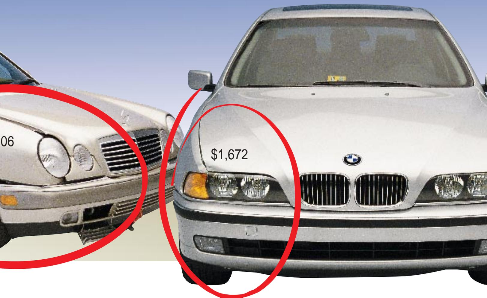
snugly against the vehicle body, leaving very little room between the body and the bumper reinforcement bar to manage impact energy. So the car body instead of the bumper must absorb much of the energy. However, the Lincoln and Cadillac have bumpers that extend far enough away from the car body to minimize damage. These cars performed best in our tests.”
