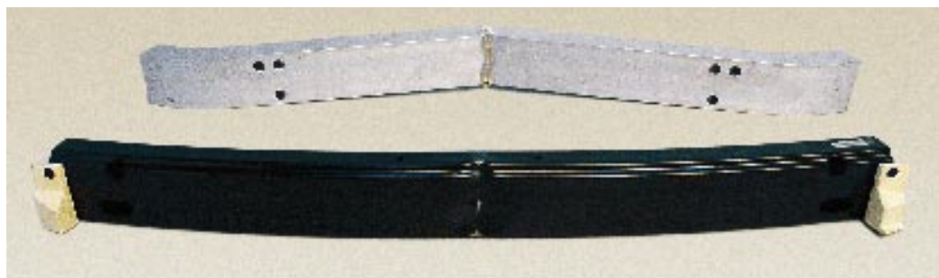
Part of what makes a good bumper is the strength of its reinforcement bar, which is hidden beneath the bumper cover. In the bottom photo, the Lexus reinforcement bar (top) bent during the rear-into-pole test at 5 mph, allowing the vehicle body to be dented as well. The Camry's reinforcement bar held up well in the rear pole test, minimizing damage to the vehicle body.
