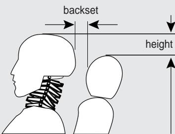
A head restraint should be at least as high as the head’s center of gravity, or about 9 centimeters (3.5 inches) below the top. The second criterion is the distance from the back of an average-size male’s head to the front of the restraint. This distance, called backset, should be small — the smaller the better. Backsets of more than 10 centimeters (about 4 inches) have been associated with increased symptoms of neck injury in crashes.
