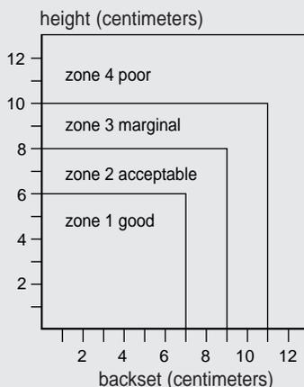
Each head restraint is classified into one of four geometric zones defined by its height and backset measures. The rating for a fixed restraint is straightforward — the zone into which its height and backset place it also defines its rating.
