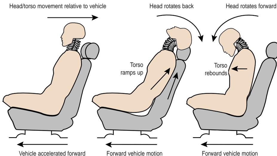
The head/neck motion of whiplash begins when a vehicle is accelerated forward by an impact. The torso moves forward after compressing the seat back, but the head lags behind. Then the head rotates rearward, bending or extending the neck back in an extension-rotation motion while the torso ramps up the seat back. Next the head and torso rebound forward. During this rebound, the head rotates forward, causing a flexed (forward-bent) neck posture before the body settles back in the seat.
