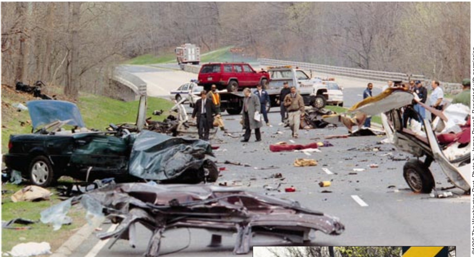
Wreckage of a four-car, head-on crash that killed three people lies scattered on the George Washington Memorial Parkway. The road lacks median barriers and has other hazards such as unprotected bridge ends (right) and trees and bridge abutments too near the roadway (below).
