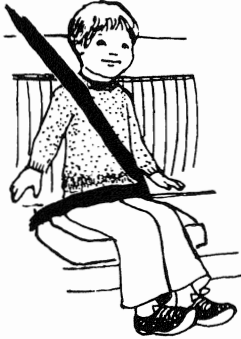
The lap belt must fit over the hips; the shoulder belt must cross the chest—not the face or neck.
