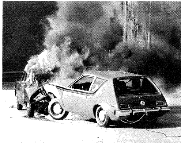
Spontaneous fire occurred in this moderate speed test crash when the gas tank ruptured.
