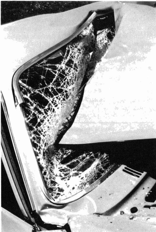
Meat Axe Effect in 1971 Vega Crash Test
