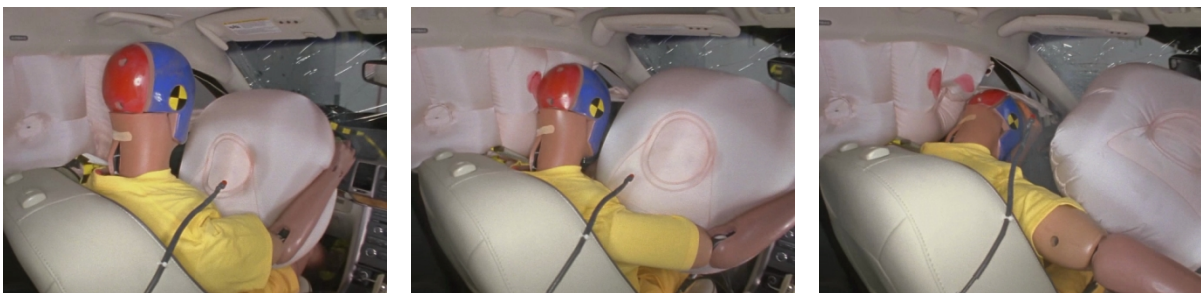
Figure 7 Example of Minimal Frontal Airbag Interaction – 2012 Lincoln MKZ (CEN1210)
