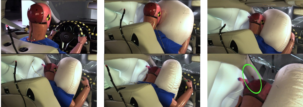
Figure 5 Example of Partial Frontal Airbag Interaction – 2014 Mercedes Benz E350 (CEN1421)
