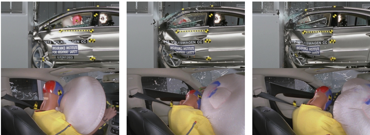
Figure 6 Example of Minimal Frontal Airbag Interaction – 2012 Volkswagen CC (CEN1203)
