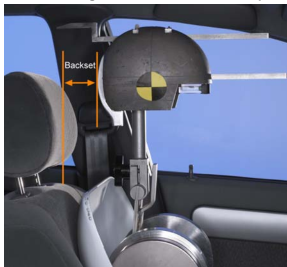
Figure 8 Measuring Backset for BioRID Set-up
