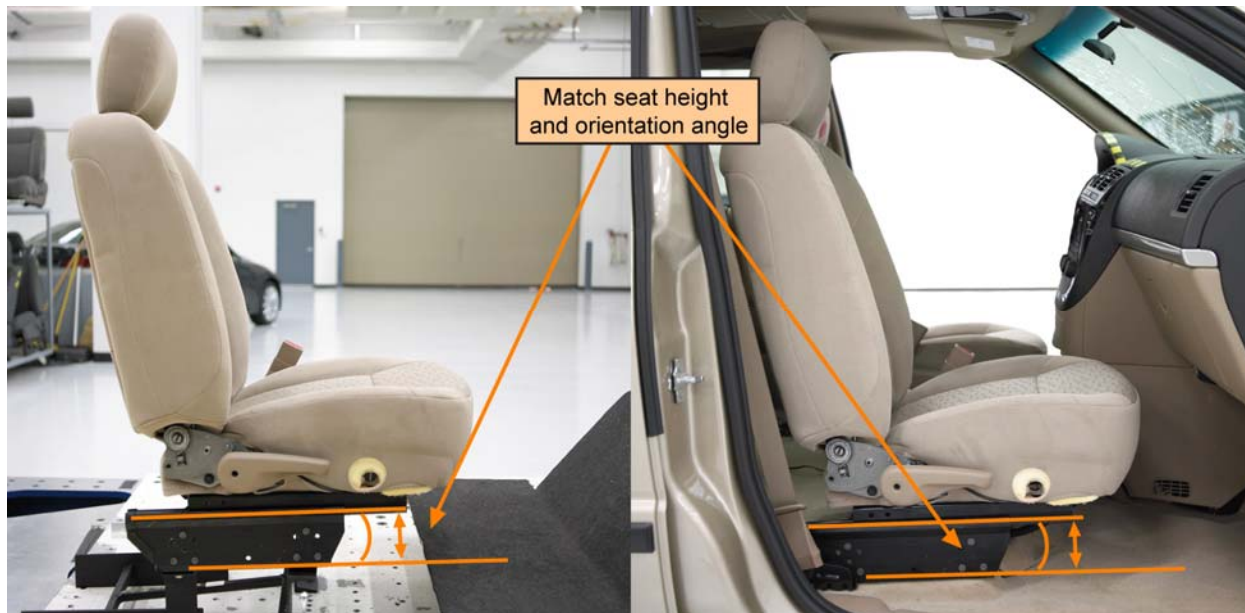
Figure 4 Attachment of Seat to Test Sled Compared with Vehicle Installation
