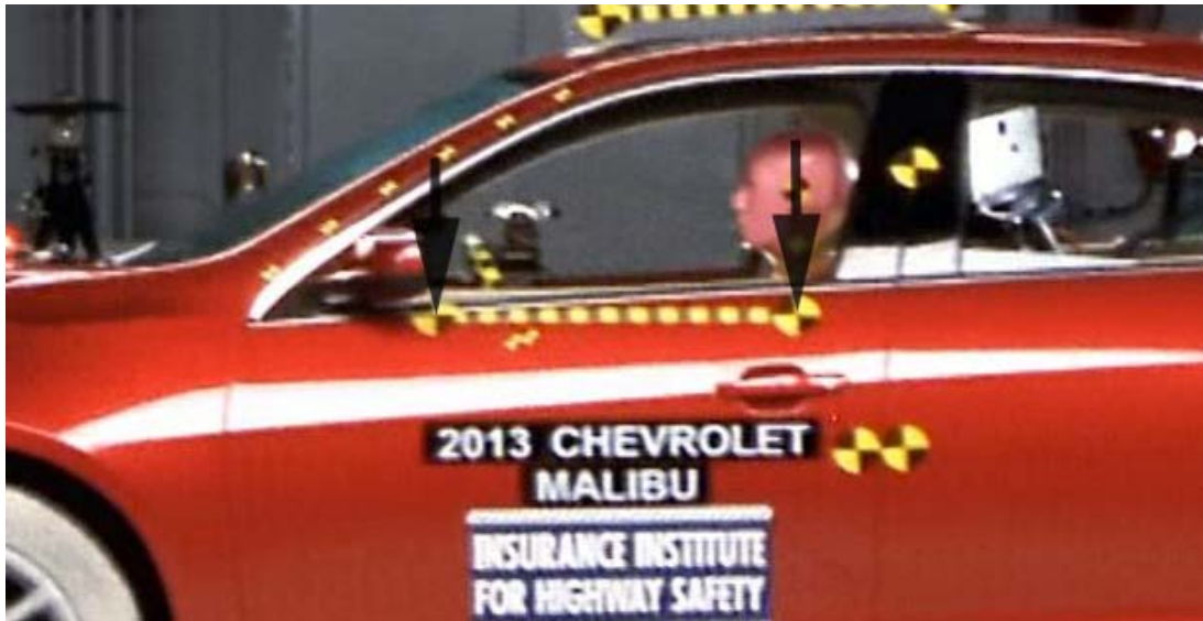
Figure 2 Distance Between Horizontal Door Targets (61 cm), All Vehicles
