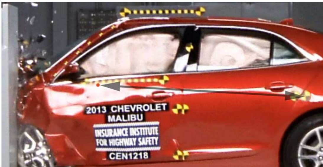
Figure 3 Marking Steering Wheel Center on Door, Mid-Crash
